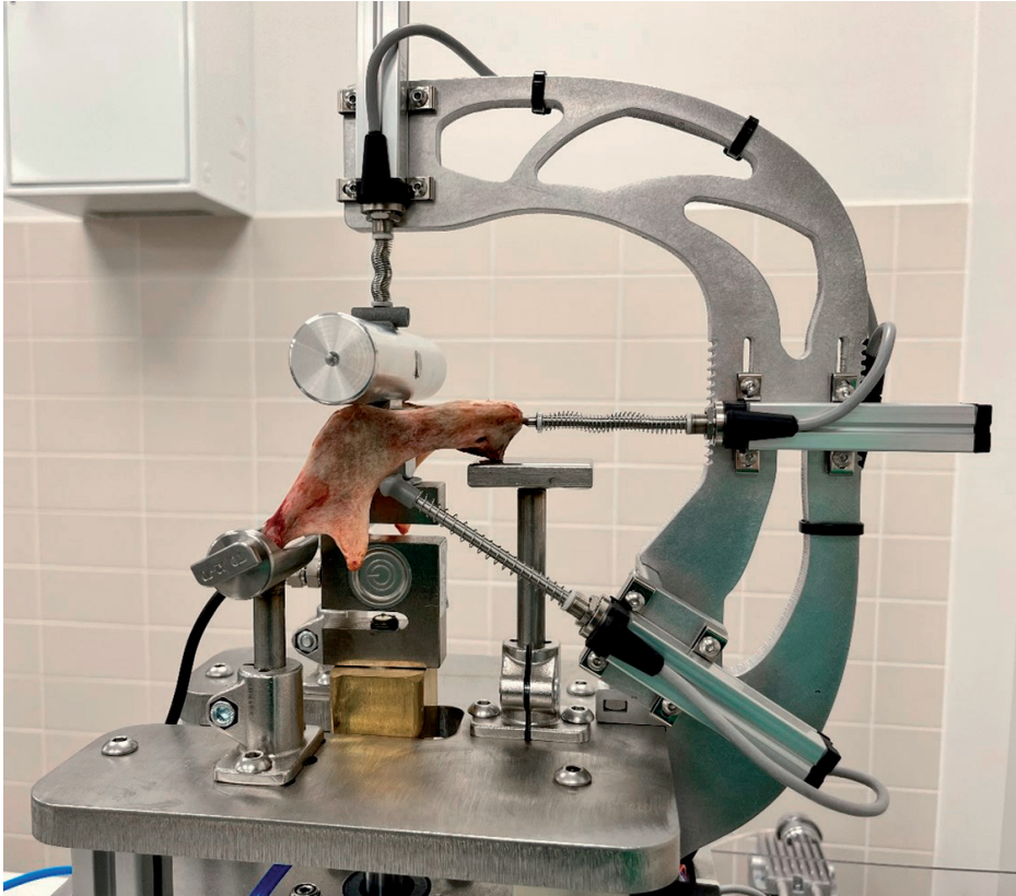
Figure 3 | A picture of the MUNACAPP apparatus ready for static uniaxial compressive testing of a cadaveric mandible.
