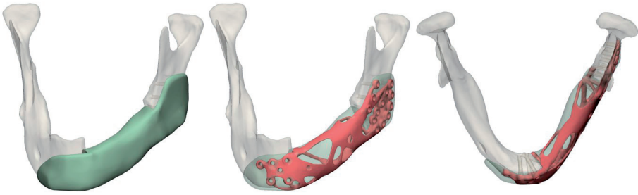
Figure 2 | An example of a topologically optimised titanium implant for the defect presented in chapter 8. The design domain is visualised in green and the final organically shaped topology optimised implant in red. The volume and weight of the design domain were reduced by 75 % though topology optimisation.
