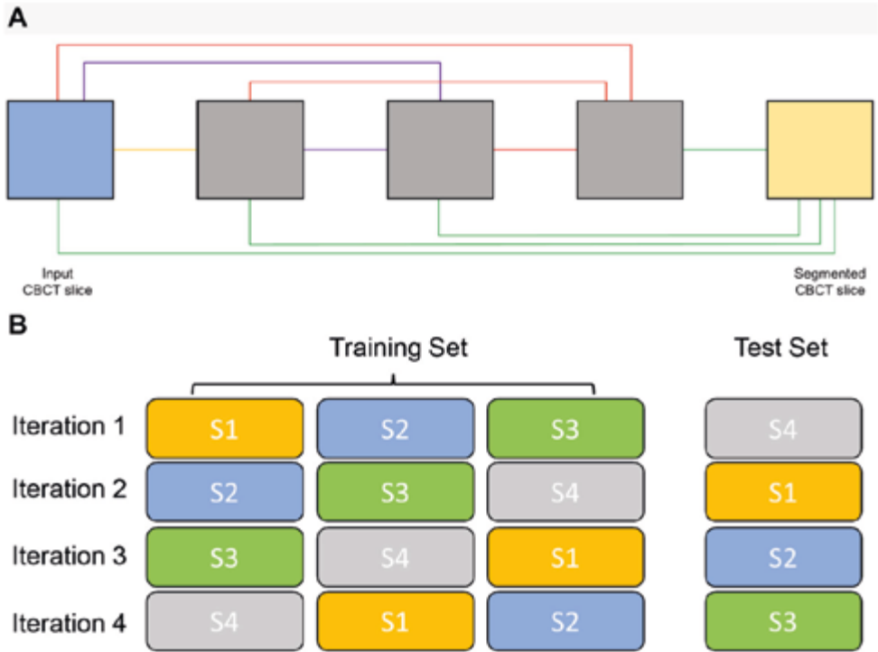
Figure 1. MS-D network architecture and 4-fold cross-validation scheme. (A) Schematic representation of an MS-D network with 3 convolutional layers and a width of 1; (B) 28 CBCT scans were divided into 4 subsets (S1, S2, S3, and S4), each containing 7 CBCT scans. For each iteration, 3 subsets were used for training and 1 for testing. CBCT, cone beam computed tomography; MS-D, mixed-scale dense.
